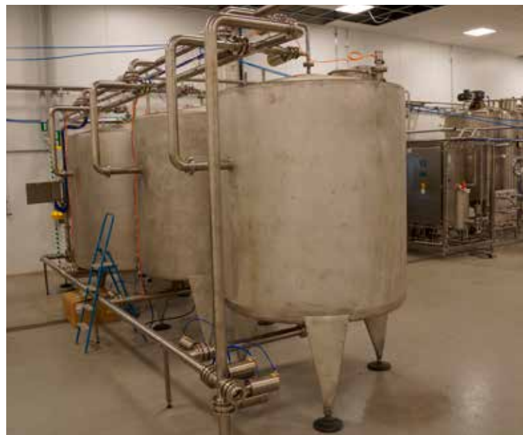
CIP unit Wellnox under installation
